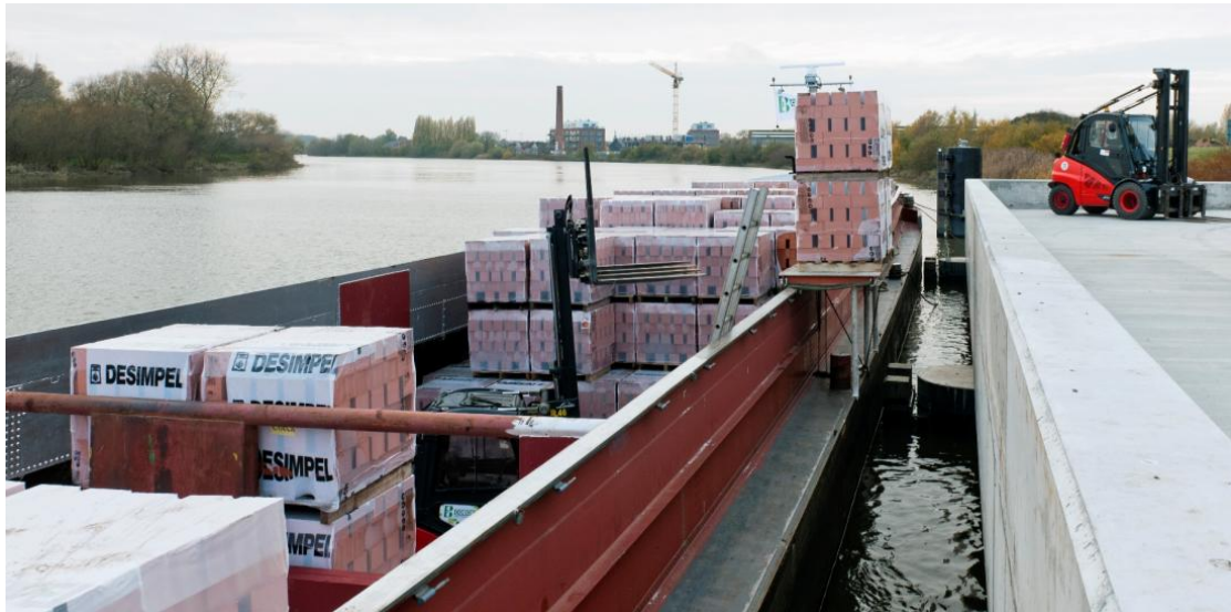
Figure 48: Loading at the Wienerberger quay in Rumst (Belgium) using two forklifts and an intermediary support structure (source: Wienerberger)
