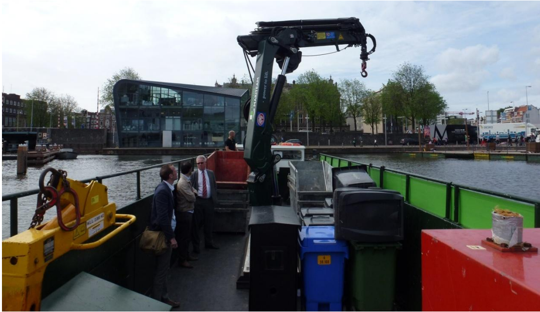
Figure 52: On-board crane on the City Supplier operated by Mokum Mariteam in Amsterdam (source: Technum)
