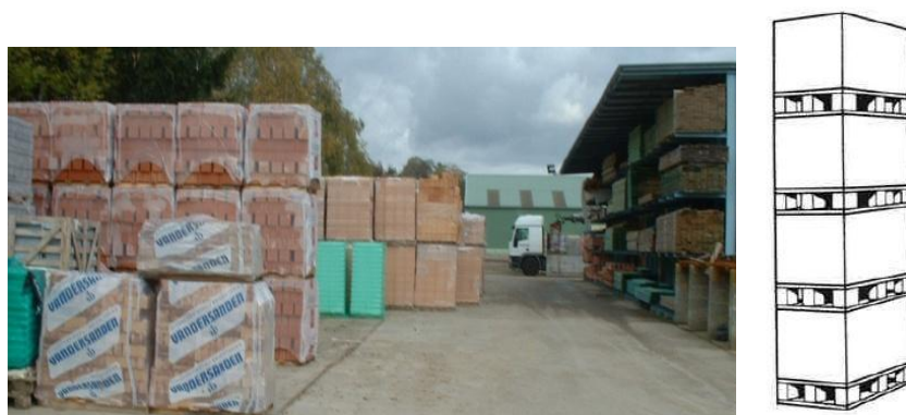
Figure 42: Pallets stacked with building blocks on 3 or 4 levels
